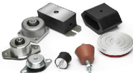
*The insulation degree (opposite of transmissibility) represents the quantity of the vibratory energy absorbed by the antivibration mount, therefore not transferred to the environment. A good percent insulation ranges from 70% to 90%.*
